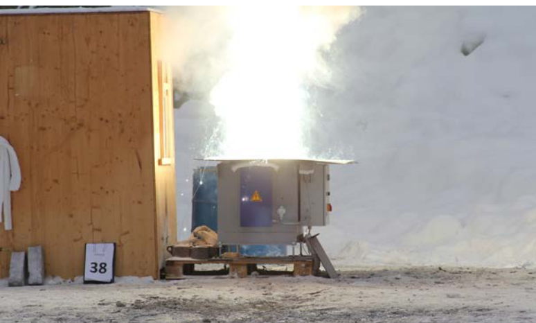
Figure 32 Molten metal ejection in case of a lithium ion accumulator (smartphone, torch)
