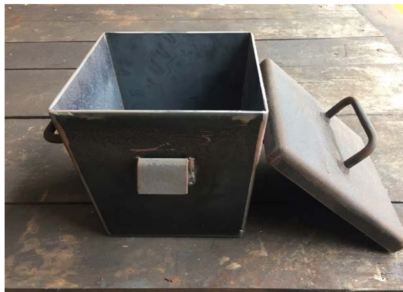
Figure 16 Dross container made of steel ...
