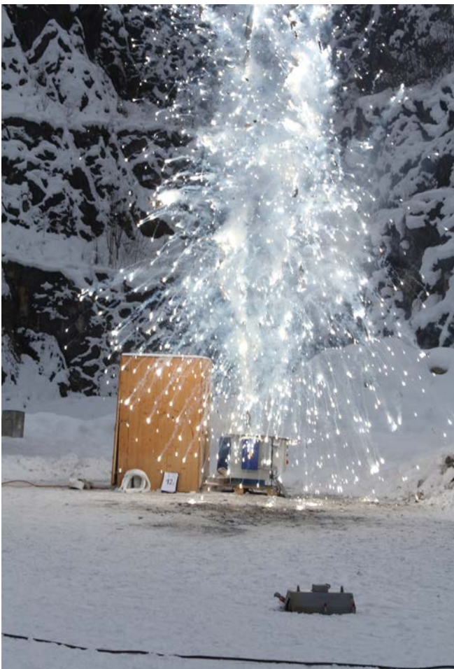
Figure 3 Thermolysis reaction of water (approx. 50 ml) added to molten magnesium
