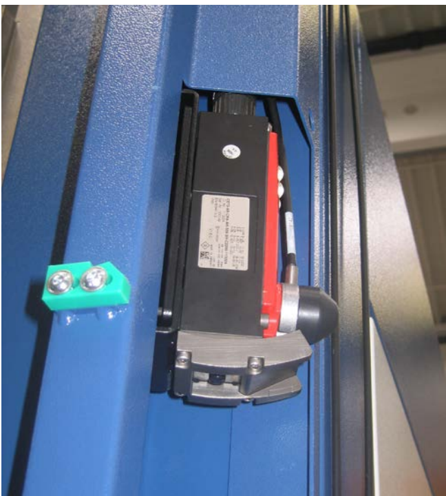
Figure 6 Interlocking guard with guard locking/position switch with emergency unlocking by Bowden cable
