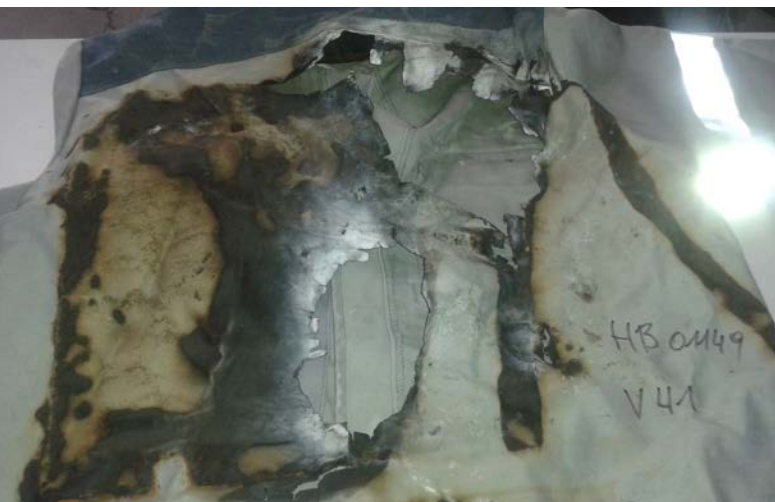
Figure 29 Burnt unsuitable protective clothing
